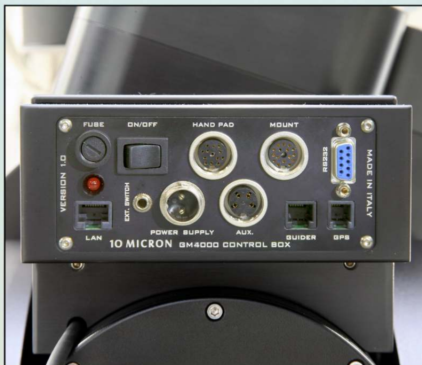
La control box sulla GM4000HPS.
